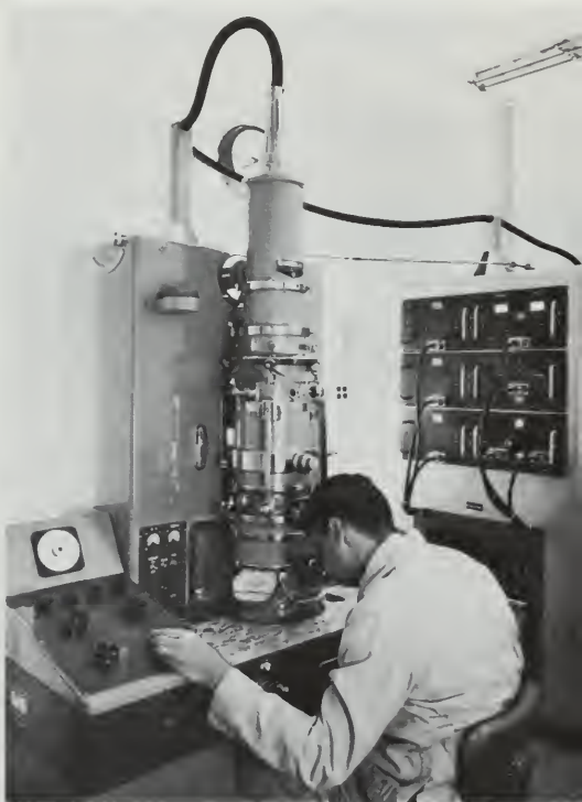
The electron microscope makes possible the study of changes in surfaces of wool fibers when a fabric is treated chemically to control shrinkage.
